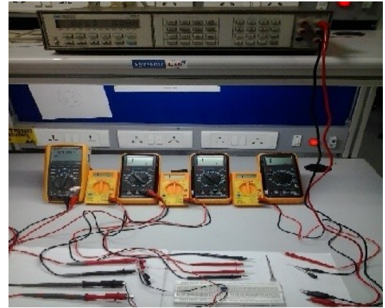
Circuit 3: Resistance benchmarking of multimeter Pic:3 Resistance benchmarking for all test multimeter FK=Fluke 287(Std. Meter), TM1=Var 0305, TM2=Var 0314, TM3=Var 0315, TM4=DT0303, TM5=DT0311, TM6=DT0323, TM7= HP 3457A.
